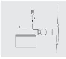
4. Fasten the screw to lock up LED Module.
