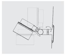
5. Adjust Dapple light projector to the desired tilt and rotation angle, lock the position.
