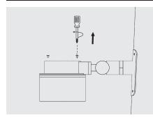
1. Unscrew to unlock the LED Module. The tilt and rotation aiming lock can left untouch.
