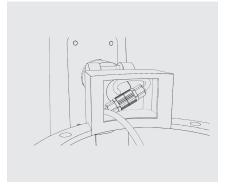
3. Push the connector into the housing.
