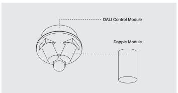
2. Each Dapple Module can be removed and exchanged. DALI Control Module can be removed and exchanged.
