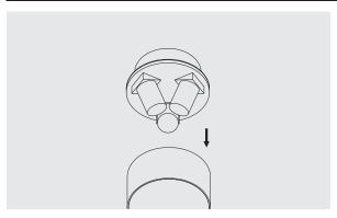
1. Unscrew and slide down front cover to expose the individual Dapple Module.
