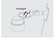
2. Unplugged the connector. The LED Module now is free. Can move to workstation to do maintenance.
