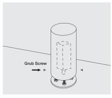
2. Install first bollard segment with 3. If necessary for increase height, LED power supplies. Secure with grub screw.
