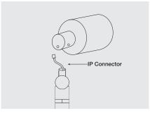
2. Unplugged the connector. The LED Module now is free. Can move to workstation to do maintenance.
