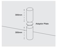
install another segment of 300mm bollard through adaptor plate.
