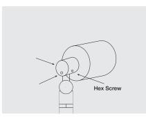
1. Unscrew to unlock the LED Module.
