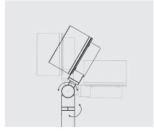
4. Adjust Dapple light projector to the desired tilt and rotation angle, lock the position.
