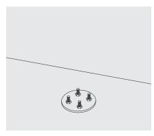
1. Secure base installation plate to pre-fab concrete slab with screw studs.
