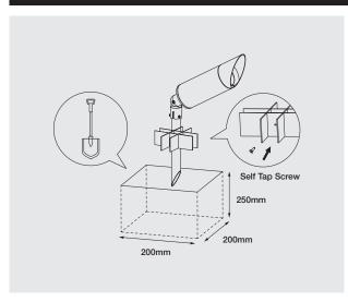
1. Dig out footing area and insert Tree Spike luminaire accordingly.
