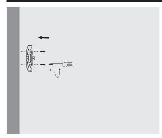
1. Install the bracket to the ceiling.
