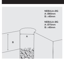
Prepare opening on concrete surface with gravel beneath for drainage.
