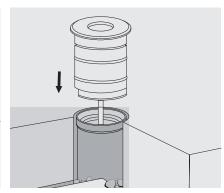
3. Insert cable through conduit and push the fixture into the embedded sleeve.
