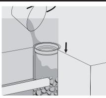
2. Insert embedded sleeve and conduit into the opening and seal with cement.
