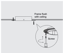
2. Secure trimless kit onto ceiling with screws.
