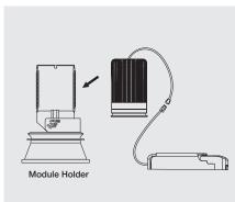
2. Attach module to module holder 3. Gently insert module holder with spring clip and connect module to driver.
