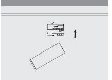
2. Attach track luminaire onto surface mounted track.
