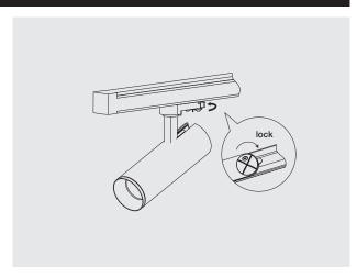
2. Secure the fixture by locking.
