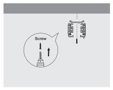
1. Secure surface mounted track onto ceiling with screw.
