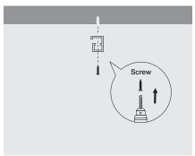
1. Secure ceiling bracket onto ceiling with screw.
