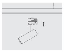
3. Attach track luminaire onto suspended track.
