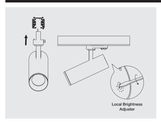
1. Adjust local brightness & attach fixture to track adapter.
