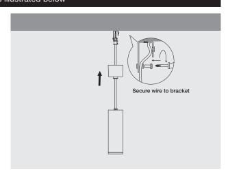
2. Connect wire & install the fixture to the ceiling.
